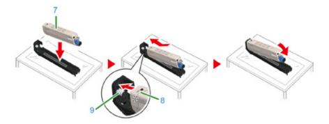
12 Turn the toner cartridge lock lever (blue) (10) of the toner cartridge backward until its top align on the ▶ mark while pressing the toner cartridge to attach the toner cartridge to the image drum.
