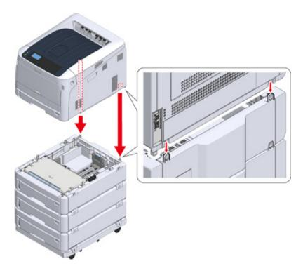
7 Join the additional tray unit to the printer unit.
