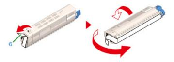
Insert a new toner cartridge (7) by aligning its left side indentation (8) with the protrusion (9) on the image drum so that the toner cartridge and image drum color label align. Then insert the right side gently into place.
