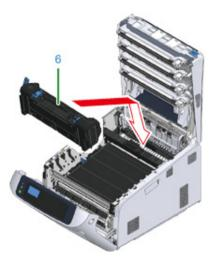
11 Push the left lock lever (5) of the fuser unit backward.
