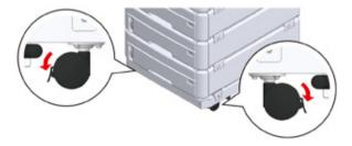
When three or more additional tray units have been attached, pull out the tipover protection tools before using the printer.
