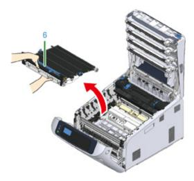
Hold the blue handle of a new belt unit, support the bottom of the belt unit, and insert the axis of the belt unit into the groove (7) in the printer.
