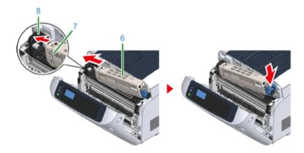
While pressing the toner cartridge, turn the toner cartridge lock lever (blue) (3) backward until its to aligns on the ▶ mark, and lock the toner cartridge to the image drum.
