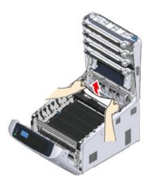
Hold the fuser unit handle (6) and place the fuser unit into the machine.
