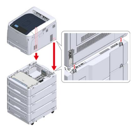
When attaching the additional tray unit, connect the printer unit and the additional tray unit.
