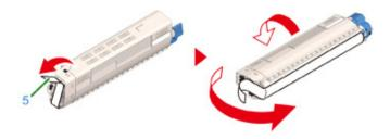
Insert a new toner cartridge (6) by aligning its left side indentation (7) with the protrusion (8) on the image drum so the toner cartridge and image drum [K] color label align. Then insert the right side gently into place.
