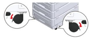
When three or more additional tray units have been attached, pull out the tipover protection tools before using the machine.
