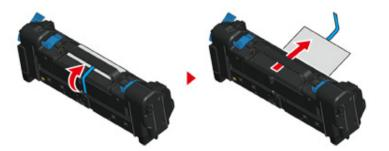
7 Pull the protective sheet in the direction of the arrow to remove.
