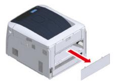
Ensure that the duplex unit is the right way up, as shown, and push it into the slot at the rear of the printer.
