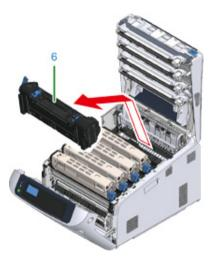
Peel off the tape from the new fuser unit, and pass the tape through the handle of the fuser unit.
