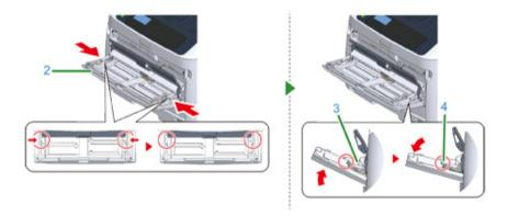
In the same manner, while pressing the left arm on the MP tray inward, slightly lift the MP tray and hook the tab.
