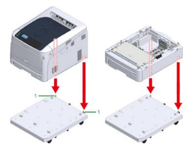
Connect the printer unit and the caster base or the additional tray unit and the caster base.
