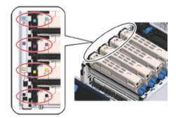
Turn the toner cartridge lock lever (blue) (5) of the toner cartridge toward you until its top align on the ▶ mark to detach the toner cartridge from the image drum.
