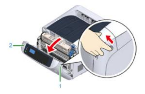
2 Remove the jammed paper gently in the direction of the arrow if an edge of jammed paper can be seen, and then go to step 8. If you cannot find jammed paper, go to step 3.
