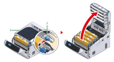
Prepare flat surface covered with sheets of newspaper, etc. to remove protective sheets from the image drums set in the printer.
