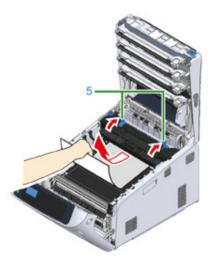
Return all four image drums into the machine carefully.
