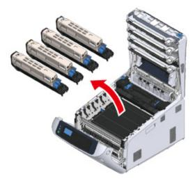
Cover the removed image drums with paper so that the image drums are not exposed to light.
