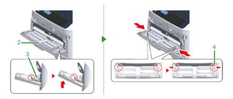
In the same manner, slightly lifting the MP tray, press the left arm inward, then unlock the tab.
