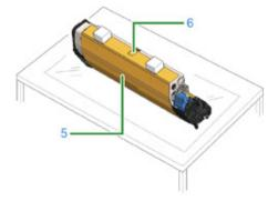
(2) Draw the protective sheet (5) in the direction of the arrow. Do not turn the toner cartridge lock lever (7) (blue).
