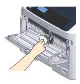
• Do not damage the paper end sensor lever when cleaning the rollers.
