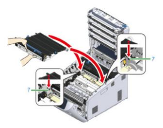
Q Lower the handle side of the belt unit and set the belt unit to the machine.
