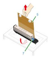
Put the image drum with the protective sheet removed into the printer unit and turn the toner cartridge lock lever (7) (blue) in the direction of the arrow until it lines up with the .
