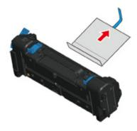
Pull forward the left locking lever (5) of the fuser unit.
