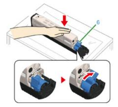
13 Check the label color of the new image drum and place the drum into the machine.
