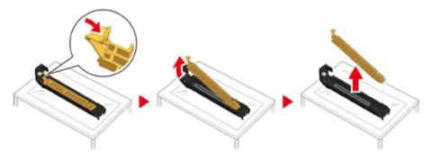
Insert the toner cartridge (7) removed in step 7 by aligning its left side indentation (8) with the protrusion (9) on the image drum so that the toner
