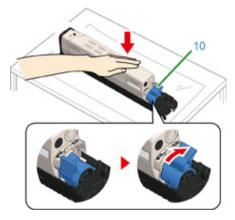
3 Check a label color of a new image drum and place the drum into the machine.
