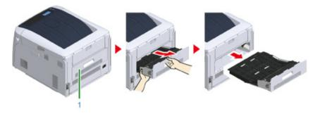
2 Check for jammed paper inside the machine. If jammed paper remains, remove it.
