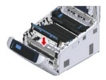
Turn the blue knobs (5) on both sides of the belt unit in the direction of the arrow to lock the belt unit.
