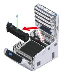
Lift the release levers (7) on the fuser unit, and pull out the jammed paper forward gently.
