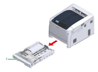
2 Set the paper size dial (2) to match the size of the paper to be loaded. Set the dial to [A4□] when loading A4 size paper in horizontal orientation.
