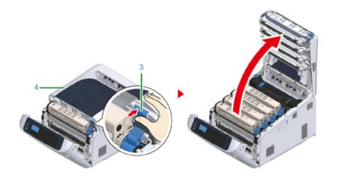
Hold the toner cartridge with both hands and pull it out along with the image drum. Pull out all 4 colors of toner cartridge and image drums, and set it on a flat surface covered with sheets of newspaper, etc.
