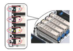
Remove the image drum (5) from the machine and place it on a flat surface.
