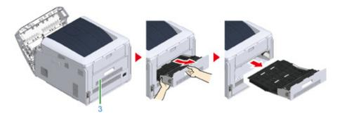
Check for jammed paper inside the machine. If jammed paper remains, remove it.
