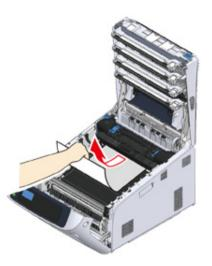
Pull out the jammed paper gently while lifting the release levers (5) on the fuser unit if an edge of jammed paper cannot be seen.
