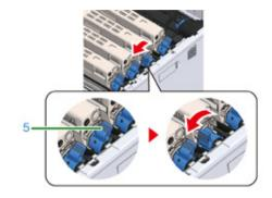
6 Lift the toner cartridge (6) from right side, and remove it from the machine.
