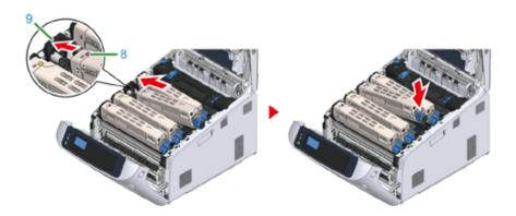
While pressing the toner cartridge, turn the toner cartridge lock lever (blue) (5) backward until its to aligns on the ▶ mark, and lock the toner cartridge to the image drum.
